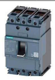
CIRCUIT BREAKER 3VA1 IEC FRAME 100 BREAKING CAPACITY CLASS S ICU=36KA @ 415 V 3-POLE, LINE PROTECTION TM210, FTFM, IN=100A OVERLOAD PROTECTION IR=100A FIXED SHORT CIRCUIT PROTECTION II=10 X IN CABLE CONNECTION
